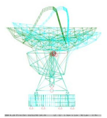
Fig. 14. Lowest eigenmode for the telescope structure. This mode has a frequency of 13.5 Hz.
