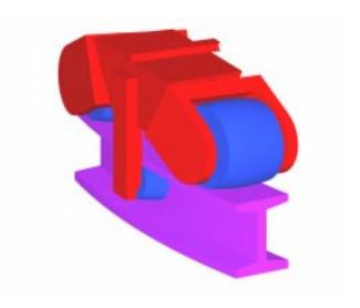
Fig. 6. Schematic of azimuth track with auto-tracking bogies.
