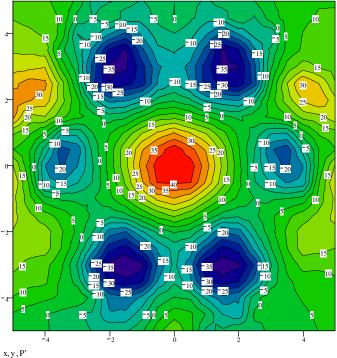
Fig. 13. Output from Mathcad analysis program with contour map for the wave front error in microns.
