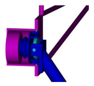
Fig. 8. Details of the elevation encoder mounting. The structure connected to the reflector nodes, including the encoder body, is shown in magenta. The structure shown in blue is part of the azimuth reference arm, including the coupler to the encoder.
