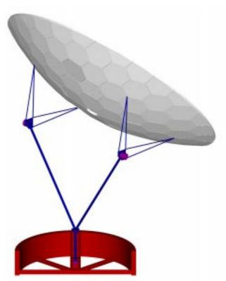
Fig. 7. Independent pointing reference structure. The CFRP beams are shown in blue and the encoders are magenta. The steel base is shown in red.
