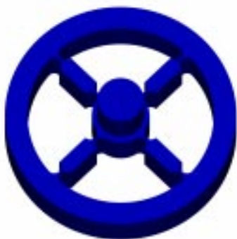
Fig. 10. Flex-pivot with high translation rigidity and low torsion stiffness for very small angles.
