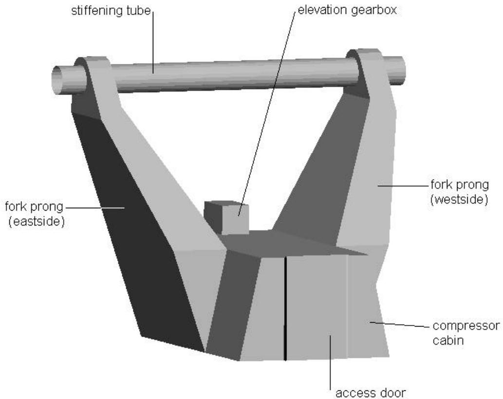
**Fig. 4.4.1:** yoke structure
