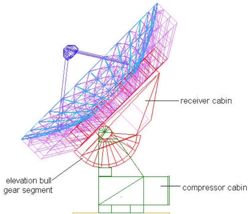
Fig. 3.2: side view on the computer model
