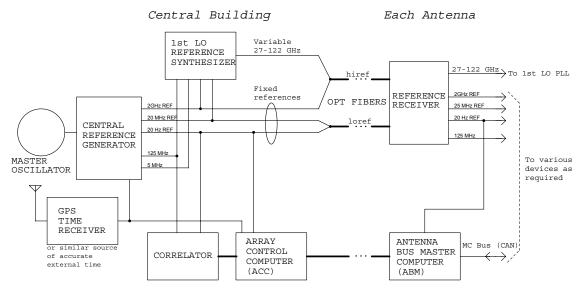
Figure 1: Simplified block diagram of the time distribution hardware.
