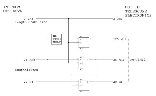
Figure 2: Ambiguity resolution circuit.
