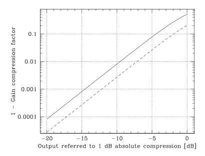
Figure 3: Gain compression factor defect limits versus output level for a device with a tanh(s) nonlinearity. The solid curve is for small differences, the dashed curve is for large signal changes.
