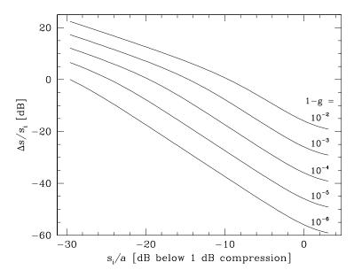
Figure 4: Gain compression error from equation (24) as a function of input signal level. Each curve represents a different gain error.
