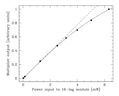
Figure 1: Compression curve for APHID's multiplier modules at a sample frequency of 1.2 GHz (points) and a least-square fit with a tanh(s) function. The dashed line is a perfectly linear response. The fitted value for the saturation factor a is 7.3 mW at the module's input.
