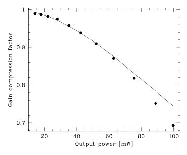
Figure 2: Measured gain compression factor with broadband noise (points) and an unconstrained plot of a  $a/s_i \tanh(s_i/a)$  function fixed to the point at a compression near 0.5 dB.
