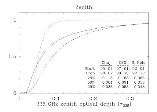
Figure 1: Cumulative distributions of the 225 GHz zenith optical depth ( $\tau_{225}$ ) measured at Chajnantor, at the CSO, and at the South Pole.
