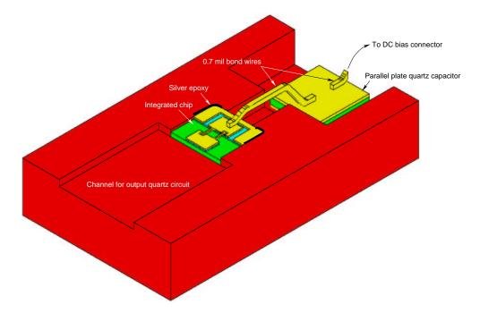
Figure E.4: Cut away view of the metal housing showing the location of the DC bias quartz capacitor and the diode chip. The location of the epoxy used to connect the ground pads to the metal housing is shown. Also shown are the 0.7 mil bond wires used to supply the DC bias to the diode chip.
