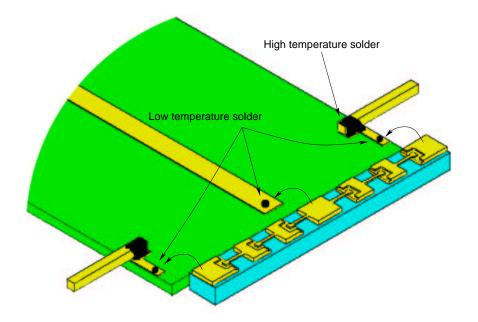
Figure E.2: Close up of the area that receives the diode array. The location of the spots with high and low temperature solder is marked. The diode is also shown placed near the location where it is to be attached.
