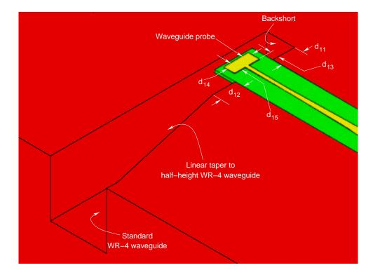
Figure 4.24: Design of the output coupler for the 80/240 GHz frequency tripler.
