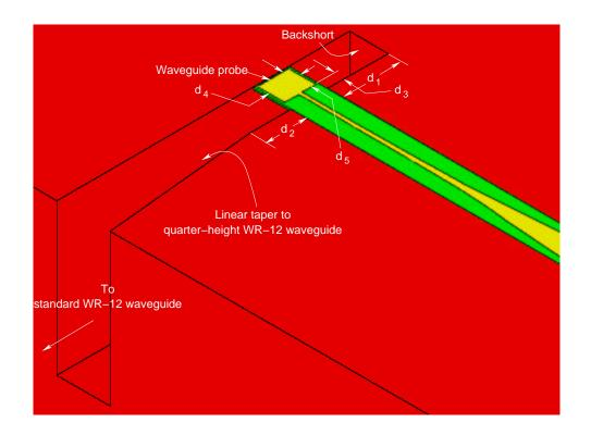
Figure 4.14: Design of the input coupler for the 80/240 GHz frequency tripler.
