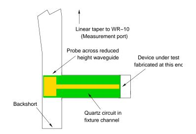
Figure 3.8: Cut away view of the test fixture, showing the placement of quartz circuit with the device under test inside.
