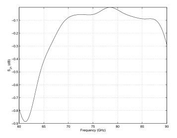
Figure 4.21: Plot of  $S_{21}$  for the complete 80/240 GHz frequency tripler input circuit (simulated).
