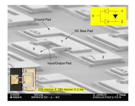
Figure 4.10: A Scanning Electron Micrograph of a completed wafer of the quartz based integrated devices, prior to the dicing operation. The location of some significant terminals is identified. The "open" diode symbols represent Schottky contacts, while the black filled diode symbol represents the location of the DC bias bypass capacitor. A photograph of a diced chip together with its dimensions is included at the bottom. Photograph courtesy Gerhard S. Schoenthal, University
