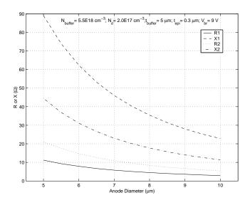
Figure 2.33: Optimum embedding impedances as a function of anode size.
