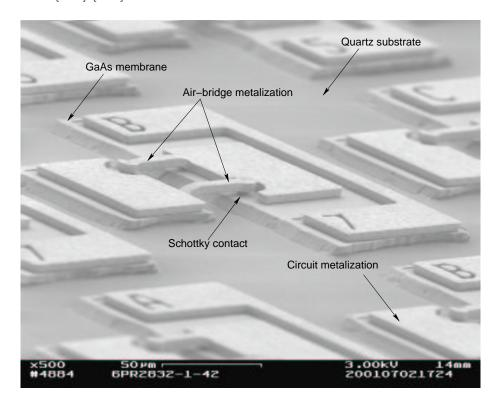
Figure 3.1: A Scanning Electron Micrograph of an undiced wafer fabricated based on the composite GaAs-membrane-on-quartz approach. Photograph courtesy Gerhard S. Schoenthal, University of Virginia, Semiconductor Development Laboratory.
