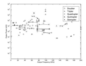
Figure 1.1: State-of-the-art frequency multiplier performance survey (1991–2001): Output power versus frequency up to 200 GHz. See Appendix-A.
