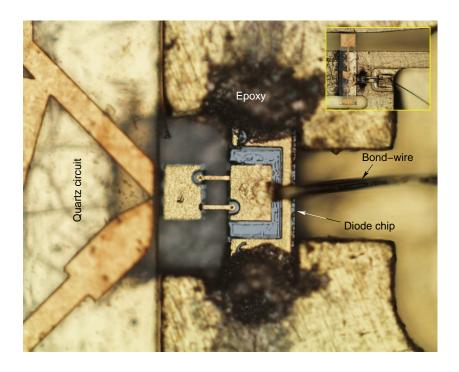
Figure E.7: Photo of the metal block showing the diode chip and the quartz circuit. A portion of the bond wire used for supplying the DC bias to the chip can be seen. The location of silver epoxy used to ground the chip pads is marked. Inset in the top right corner is an overall view of the block showing the entire quartz circuit seated next to the diode chip. The quartz DC bias capacitor as well as the 0.7 mil diameter bond wires can also be seen.
