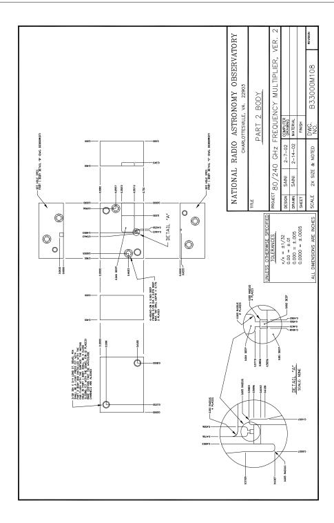
Figure D.48: 80/240 GHz frequency tripler, version 2: Mechanical details of part 2 of the two piece split block.
