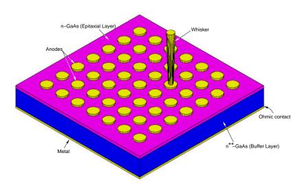
Figure A.1: Whisker contacted abrupt junction Schottky diode.
