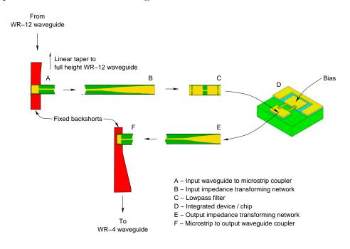
Figure 4.4: Relative placement of various components used in the 80/240 GHz frequency tripler.
