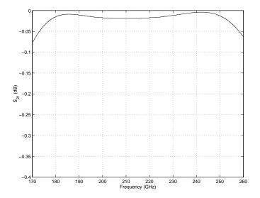
Figure 4.26: Plot of  $S_{21}$  for the output 50  $\Omega$  microstrip to WR-4 waveguide transition (simulated).
