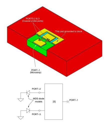
Figure 4.11: Cut away view of the structure analyzed in HP-HFSS to compute the S-parameters of the frequency tripler chip. Only bottom half of the mount that seats the diode chip is shown. Also shown at the bottom is the equivalent circuit model schematic (based on the calculated S-parameters) used in MDS to perform harmonic balance simulations to calculate the optimum input and output embedding impedances. For simplicity, the DC bias arrangement has been omitted and is not shown.
