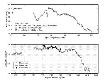
Figure 4.38: Performance of the modified 80/240 GHz frequency tripler built using a diode chip having 6  $\mu m$  diameter anodes, with the DC bias bypass capacitor shorted to the ground pad with silver epoxy.
