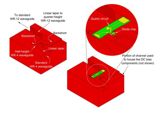
Figure 4.34: The modified 80/240 GHz frequency tripler. Figure shows a cutaway view of the split block mount revealing the location of the planar quartz circuit and the placement of the diode chip alongside it. The DC bias components and bond wires are omitted.
