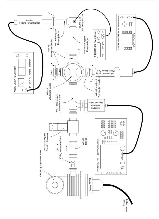
Figure 2.25: Experimental setup for evaluation of the 55/110 GHz frequency doubler.
