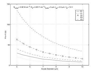
Figure 4.9: Optimum embedding impedances as a function of anode size.
