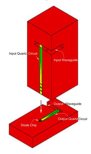
Figure E.5: Cut away view of the relevant pieces of the metal housing showing the relative placement of the diode chip, the input quartz circuit and the output quartz circuit. The DC bias arrangement located adjacent to the diode chip is not shown.
