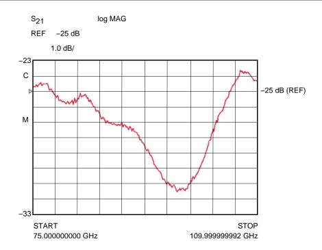
Figure 3.12: Plot of the measured values of  $S_{21}$  for the spiral inductor structure of Figure-3.10.
