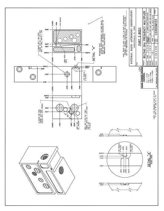
Figure D.43: 80/240 GHz frequency tripler, version 1: Mechanical details of part 3 of the three piece metal block.
