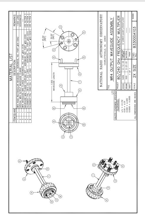
Figure D.39: 80/240 GHz frequency tripler, version 1 and 2: WR-4 output waveguide flange adapter assembly.
