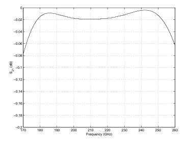
**Figure 3.6:** Plot of  $S_{21}$  for the microstrip to WR-4 waveguide transition of Figure-3.4.
