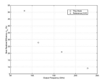
Figure 2.41: Plot of the best reported and measured efficiencies of various frequency doublers built based on the hybrid approach.
