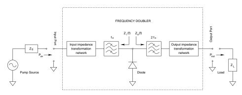
Figure 2.1: A single diode based frequency doubler.
