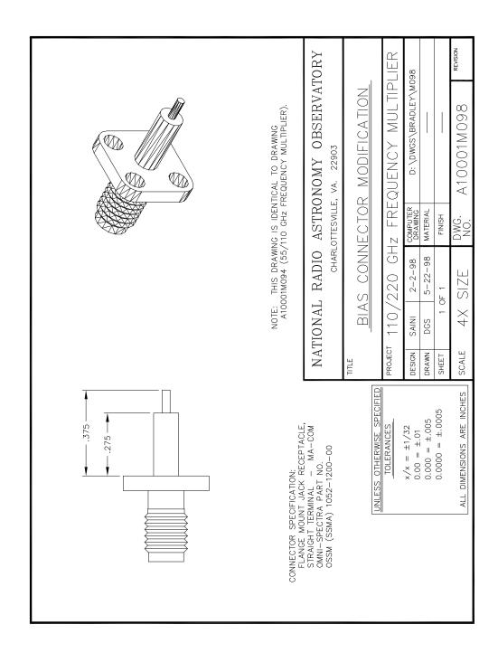
Figure D.35: 110/220 GHz frequency doubler: Details of the modified SSMA flange mount jack receptacle used as the DC bias connector.
