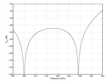
Figure 2.35: Plot of  $S_{21}$  for the DC bias filter (simulated).
