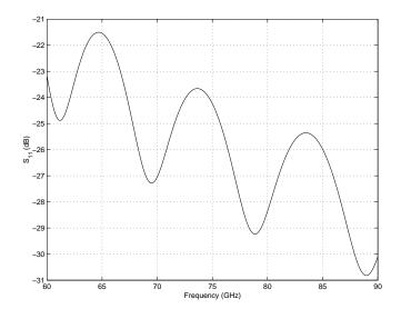
Figure 4.13: Plot of  $S_{11}$  for the WR-12 one-fourth to full height waveguide linear taper (simulated).
