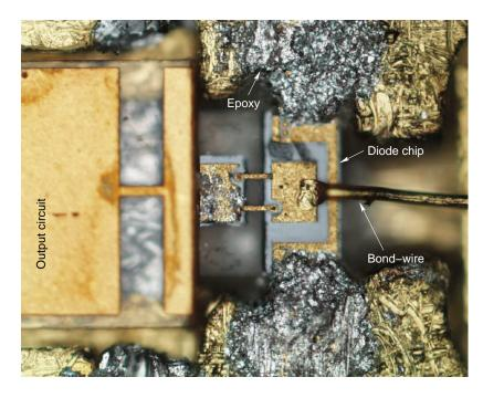
Figure E.6: Photo of the metal block showing the diode chip and the output circuit. A portion of the bond wire used for supplying the DC bias to the chip can be seen. The location of silver epoxy used to ground the chip pads is marked.
