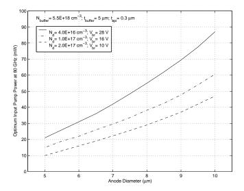
Figure 4.7: Input power (per diode) to obtain maximum conversion efficiency, for different anode sizes and epitaxial layer doping level.
