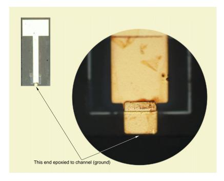
Figure 3.7: Photograph of 2 mil thick quartz circuit showing the test capacitor at one end of the microstrip transmission line. The waveguide probe is visible as a "flag" structure on the other end of the microstrip.
