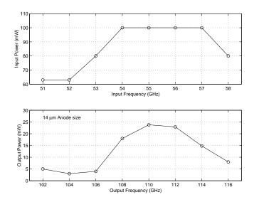
Figure 2.29: Plot of the measured output power versus frequency for the 55/110 GHz frequency doubler using a diode array with 14  $\mu m$  diameter anodes.
