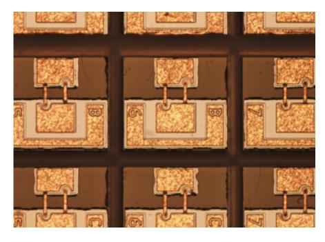
Figure 3.2: Photograph of the diced wafer prior to backside lapping to achieve chip separation. Photograph courtesy Gerhard S. Schoenthal, University of Virginia, Semiconductor Development Laboratory.
