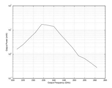
Figure 4.30: Calculated output power of the 80/240 GHz frequency tripler as a function of output frequency.
