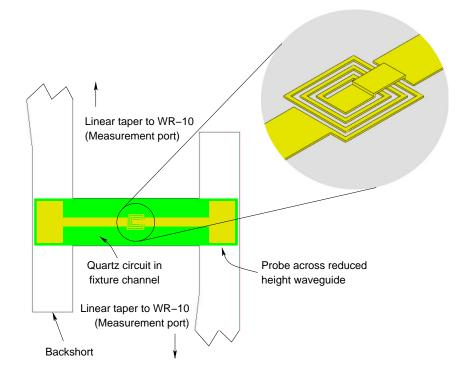
Figure 3.10: The circuit used for the evaluation of the planar integrated inductor element [154].
