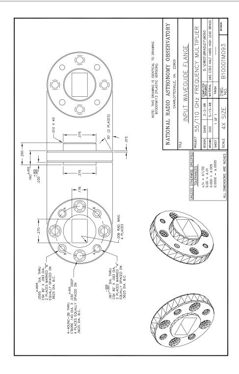
Figure D.14: 55/110 GHz frequency doubler: Mechanical details of the special WR-19 input waveguide flange.
