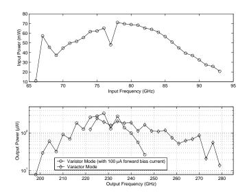
Figure 4.33: Measured performance of the 80/240 GHz frequency tripler, built using a diode chip having 6  $\mu m$  diameter anodes.
