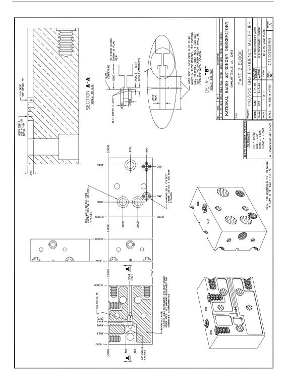
Figure D.33: 110/220 GHz frequency doubler: Mechanical details of part 2 of the two piece split block.
