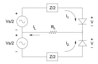
Figure 2.2: An alternate doubler circuit employing a balanced diode configuration.
