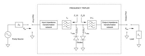
Figure 4.3: A practical frequency tripler circuit configuration based on antiparallel arrangement of diodes.
