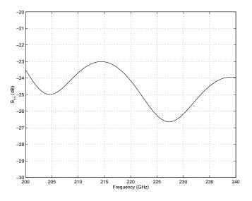
Figure 2.36: Plot of  $S_{11}$  for the WR-4 one-fifth to full height waveguide linear taper (simulated).
