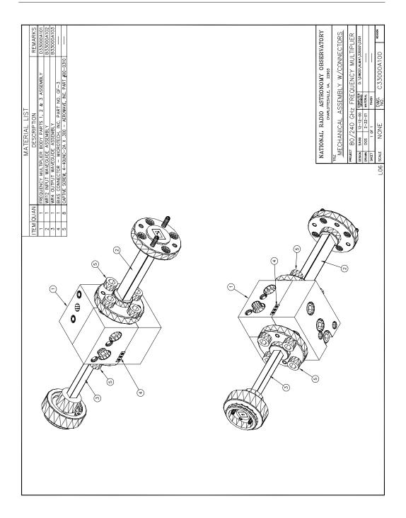
**Figure D.36:** 80/240 GHz frequency tripler, version 1: Mechanical assembly of the three piece block showing the DC bias connector and the waveguide flange adapters.
