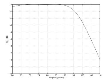
**Figure 4.18:** Plot of  $S_{21}$  for the input lowpass filter (simulated).
