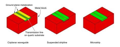
Figure 3.3: Planar transmission line structures.
