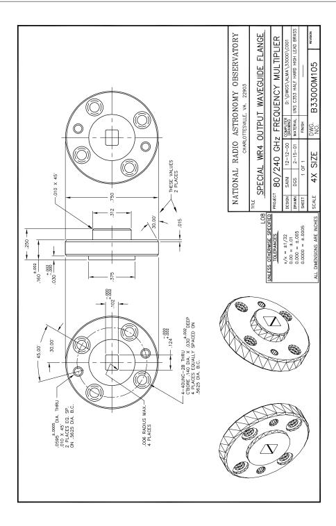
Figure D.45: 80/240 GHz frequency tripler, version 1 and 2: Mechanical details of the special WR-4 output waveguide flange.
