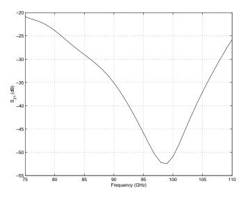
Figure 3.11: Plot of the simulated values of  $S_{21}$  for the spiral inductor structure of Figure-3.10.
