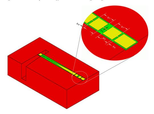
Figure 4.17: Design of the input lowpass filter. Only bottom part of the mount that seats the quartz circuit is shown. All the dimensions that were optimized are marked.
