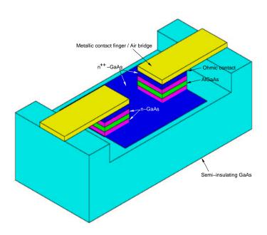
Figure A.4: Planarized hetero-junction barrier varactor diode.
