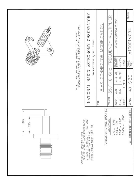
Figure D.15: 55/110 GHz frequency doubler: Details of the modified SSMA flange mount jack receptacle used as the DC bias connector.
