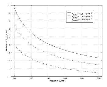
Figure 4.6: Plot of skin depth in the buffer layer vs. frequency for three doping levels.
