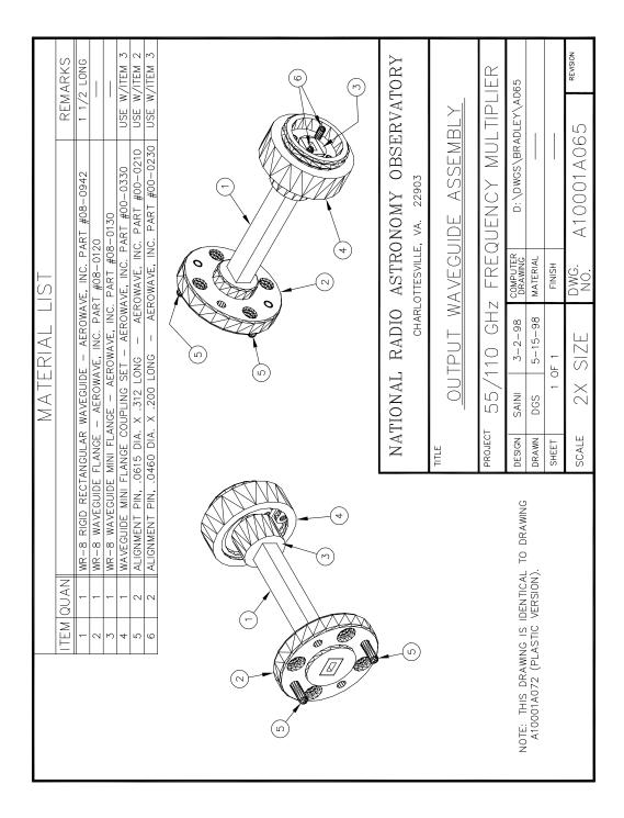
Figure D.5: 55/110 GHz frequency doubler: WR-8 output waveguide flange adapter assembly.
