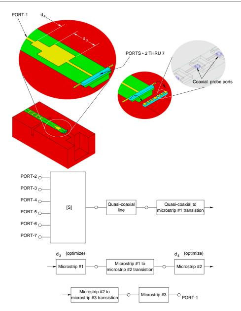
Figure 2.18: Design optimization of the impedance matching sections of the output embedding circuit for the 55/110 GHz frequency doubler. Only bottom half of the mount that seats the quartz circuit is shown. The location of various ports as well as the dimensions that were optimized are illustrated. The equivalent circuit model schematic (based on the S-parameter files generated by HP-HFSS) used in MDS to optimize the lengths  $d_3$  and  $d_4$  in the output circuit is shown at the bottom.
