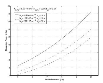
Figure 2.31: Power dissipated (per diode) under conditions of optimum operation for different anode sizes and epitaxial layer doping level.
