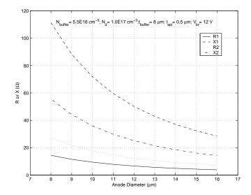
Figure 2.14: Optimum embedding impedances as a function of anode size.
