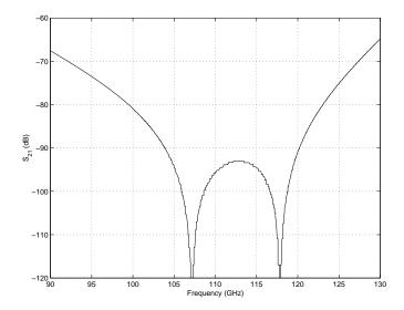
Figure 2.20: Plot of  $S_{21}$  for the DC bias filter (simulated).
