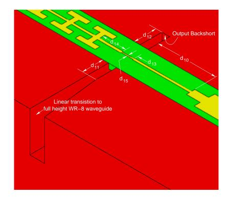
Figure 2.22: Design of the output cross-guide coupler for the 55/110 GHz frequency doubler. Only bottom half of the mount that seats the quartz circuit is shown. The dimensions that were optimized to achieve a good coupling efficiency are marked.
