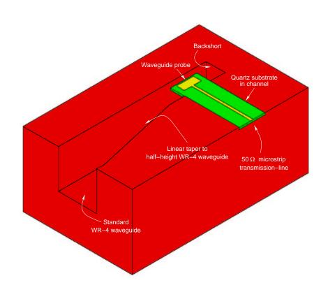
Figure 3.4: The microstrip to WR-4 waveguide transition. Figure shows a cutaway view of the arrangement. Only the bottom half of the block is illustrated, revealing the placement of the quartz circuit in the metal housing.
