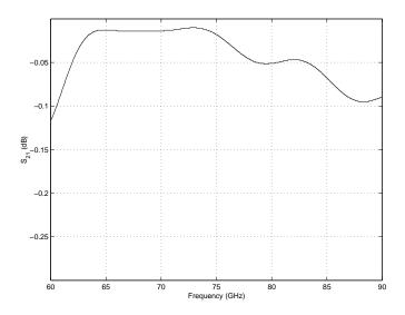
Figure 4.16: Plot of  $S_{21}$  for the input WR-12 waveguide to 50  $\Omega$  microstrip transition (simulated).
