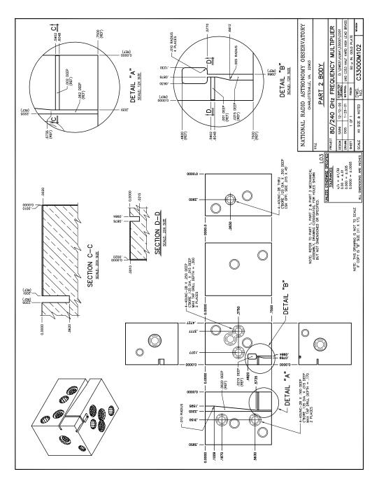
Figure D.42: 80/240 GHz frequency tripler, version 1: Mechanical details of part 2 of the three piece metal block.
