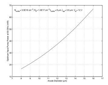
Figure 2.13: Input power (per diode) to obtain maximum conversion efficiency for a range of anode sizes for the chosen material system.
