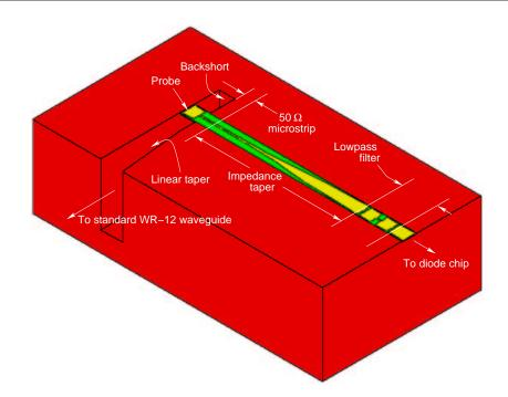
Figure 4.12: The input embedding circuit consisting of a waveguide to microstrip transition, a microstrip impedance taper and a lowpass filter. Only the bottom part of the mount that seats the quartz circuit is shown.
