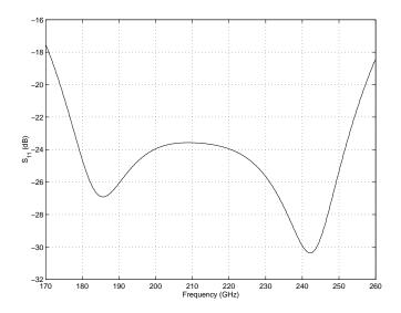
Figure 4.25: Plot of  $S_{11}$  for the output 50  $\Omega$  microstrip to WR-4 waveguide transition (simulated).
