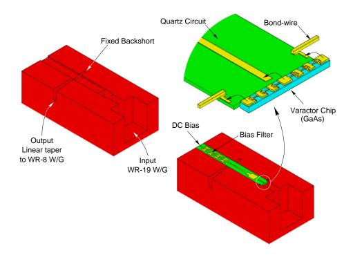
Figure 2.3: The 55/100 GHz frequency doubler. Figure shows a cut-away view of the doubler mount revealing the location of the planar quartz circuit and the placement of the diode array on it.
