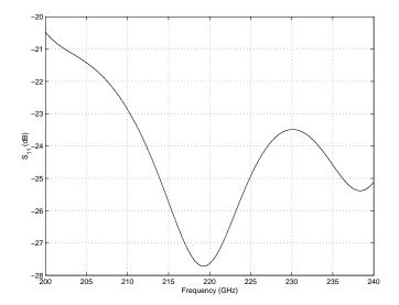
Figure 2.37: Plot of  $S_{11}$  for the complete output coupling arrangement, including the microstrip to one-fifth height waveguide probe, DC-bias filter and the one-fifth
