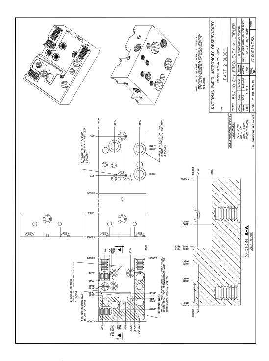
Figure D.9: 55/110 GHz frequency doubler: Mechanical details of part 2 of the two piece split block.
