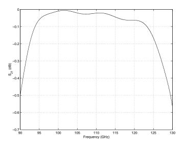
Figure 2.24: Plot of  $S_{21}$  for the complete output coupling arrangement, including the microstrip to one-fifth height waveguide probe, DC-bias filter and the one-fifth height to full height taper (simulated).
