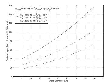
Figure 2.10: Input power (per diode) to obtain maximum conversion efficiency, for different anode sizes and epitaxial layer doping level.
