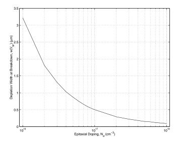
Figure 2.12: Variation of the width of the depleted region in the epitaxial layer at before breakdown as a function of epitaxial doping level.
