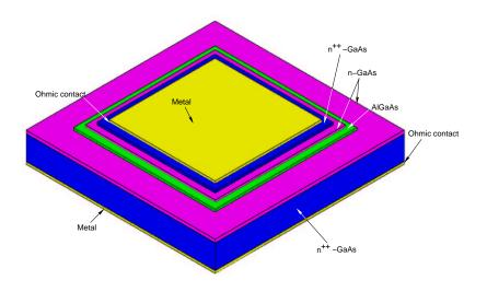
Figure A.3: Discrete hetero-junction barrier varactor diode.
