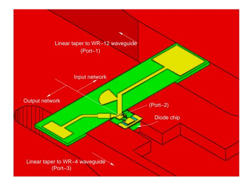
Figure 4.35: Layout of the input and output embedding circuits, integrated onto a single quartz substrate. Also illustrated is the placement of the quartz circuit relative to important features on the metal block as well as the diode chip. Only
