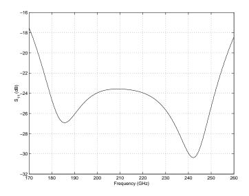
Figure 3.5: Plot of  $S_{11}$  for the microstrip to WR-4 waveguide transition of Figure-3.4.
