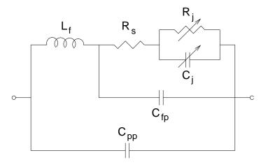
Figure 2.8: Equivalent circuit model of a Schottky junction varactor diode.
