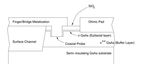
Figure 2.16: The coaxial probe geometry employed to calculate the impedance at the location of the Schottky junctions.
