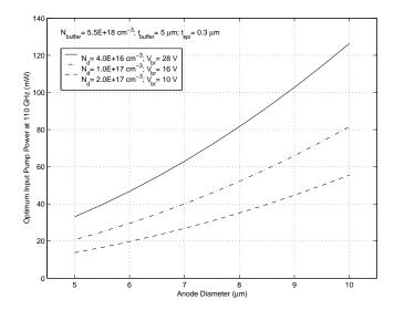
Figure 2.30: Input power (per diode) to obtain maximum conversion efficiency, for different anode sizes and epitaxial layer doping level.
