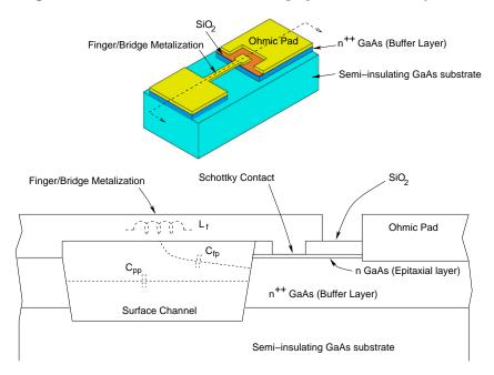
Figure A.2: Planarized abrupt junction Schottky diode.
