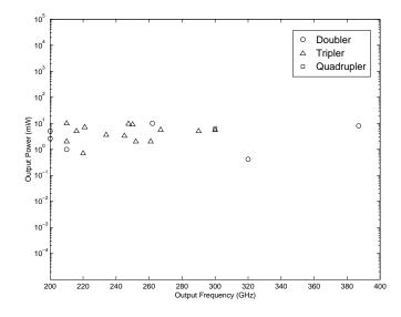
**Figure 1.2:** State-of-the-art frequency multiplier performance survey (1991–2001): Output power versus frequency from 200 GHz to 400 GHz. See Appendix-A.
