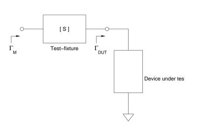
$$Z_{DUT} = 50 \left(\frac{1 + \Gamma_{DUT}}{1 - \Gamma_{DUT}}\right)$$
