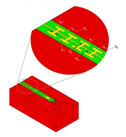
Figure 2.19: Design of the bias filter. Only bottom half of the mount that seats the quartz circuit is shown. All the dimensions that were optimized are marked.
