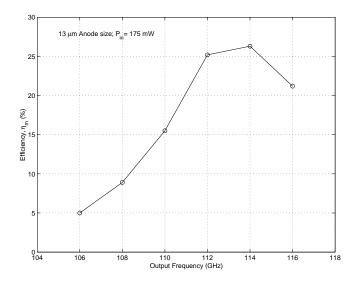
Figure 2.26: Measured conversion efficiency of the 55/110 GHz frequency doubler using a diode array with 13  $\mu m$  diameter anodes.
