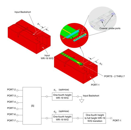
Figure 2.17: Design of the input embedding circuit for the 55/110 GHz frequency doubler. Only bottom half of the mount that seats the quartz circuit is shown, with and without the quartz circuit in place. The location of various ports as well as the dimensions that were optimized are illustrated. The equivalent circuit model schematic (based on the S-parameter files generated by HP-HFSS) used in MDS to optimize the lengths  $d_1$  and  $d_2$  in the input circuit is shown at the bottom.
