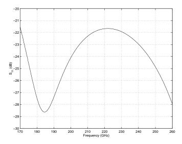
Figure 4.23: Plot of  $S_{11}$  for the WR-4 half height to full height waveguide linear taper (simulated).
