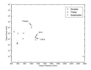
Figure 1.3: State-of-the-art frequency multiplier performance survey (1991–2001): Output power versus frequency from 400 GHz to 2600 GHz. See Appendix-A.
