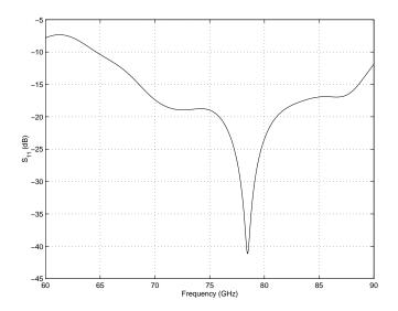
Figure 4.20: Plot of  $S_{11}$  for the complete 80/240 GHz frequency tripler input circuit (simulated).
