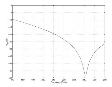
Figure 4.37: Plot of  $S_{21}$  for the modified 80/240 GHz frequency tripler quartz circuit showing the isolation provided by the radial stub in the input circuit to the third harmonic signals (simulated).
