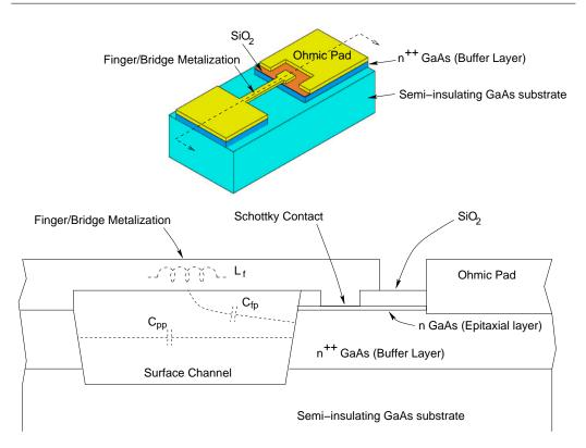
Figure 2.4: Details of a planar Schottky varactor.
