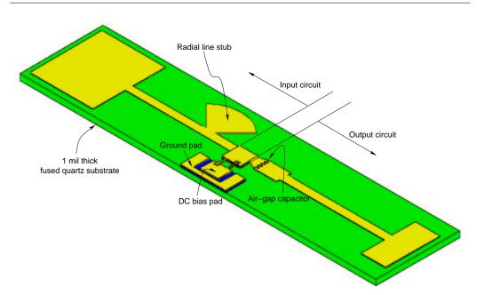
**Figure 4.39:** Layout of the 80/240 GHz frequency tripler as a MMIC chip. The embedding circuits may be fabricated integrally as shown on the extended GaAs-membrane-on-quartz substrate after the removal of GaAs from appropriate regions.
