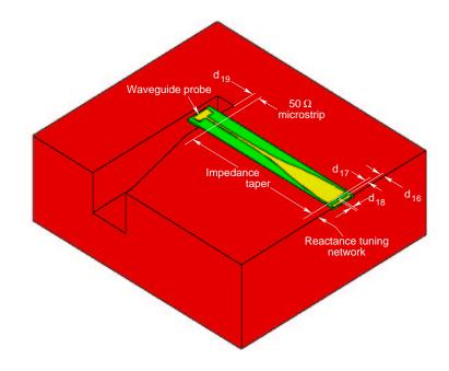
Figure 4.27: The output embedding circuit consisting of a reactance tuning structure followed by a microstrip impedance taper and a microstrip to waveguide transition. Only the bottom part of the mount that seats the quartz circuit is shown. The length of the section marked  $d_{16}$  was optimized such that the impedance presented to the diode chip was close to an open circuit at the input frequency of 80 GHz.
