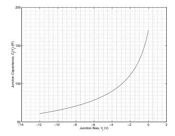
Figure 2.7: Typical variation of the varactor junction capacitance with an applied (reverse) bias voltage.
