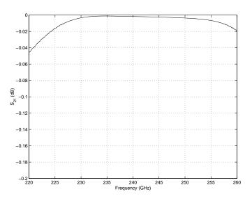
Figure 4.29: Plot of  $S_{21}$  for the complete 80/240 GHz frequency tripler output circuit (simulated).
