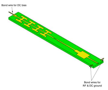
Figure E.1: Bond wire locations on the 55/110 GHz frequency doubler quartz circuit.
