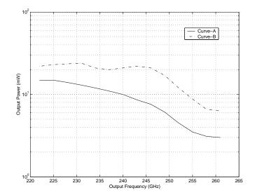
Figure 4.31: Calculated output power of the 80/240 GHz frequency tripler with the mutual loading effects between the input and output circuits ignored (curve-A). Curve-B shows the calculated output power with nearly ideal embedding impedances.
