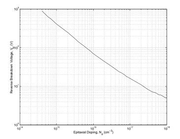
Figure 2.6: Reverse breakdown voltages as a function of epitaxial layer doping level.
