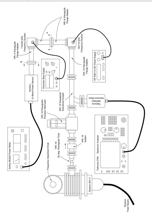
Figure 2.39: Experimental setup for evaluation of the 110/220 GHz frequency doubler.
