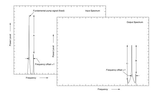
Figure 5.2: Sketches illustrate the power spectrum of the test input signal used in two-tone harmonic balance simulations (left) and the typical resulting output power spectrum (right).
