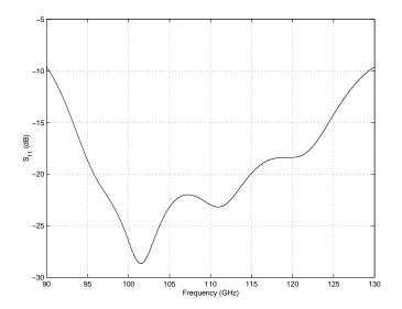
Figure 2.23: Plot of  $S_{11}$  for the complete output coupling arrangement, including the microstrip to one-fifth height waveguide probe, DC-bias filter and the one-fifth height to full height taper (simulated).
