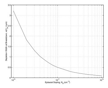
Figure 4.8: Variation of the width of the depleted region in the epitaxial layer at before breakdown as a function of epitaxial doping level.
