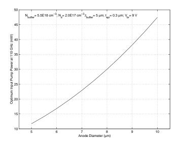
Figure 2.32: Input power (per diode) to obtain maximum conversion efficiency for a range of anode sizes for the chosen material system.
