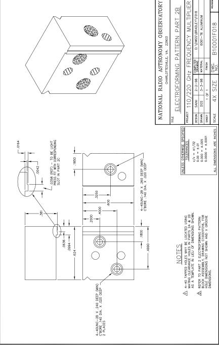
Figure D.27: 110/220 GHz frequency doubler: Mechanical details of the mandrel
