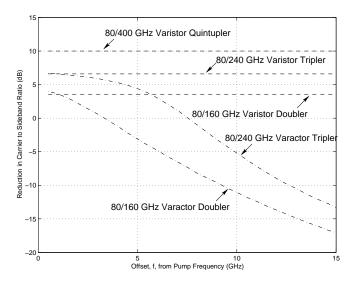
Figure 5.4: Plot of the degradation in carrier-to-sideband ratio for various frequency multipliers.
