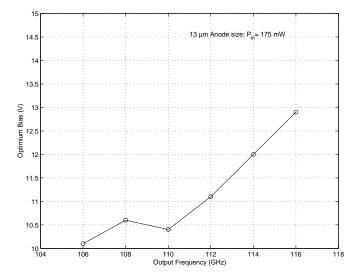
Figure 2.27: Plot of the measured optimum bias voltage versus output frequency.
