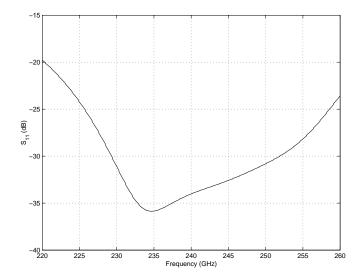
Figure 4.28: Plot of  $S_{11}$  for the complete 80/240 GHz frequency tripler output circuit (simulated).
