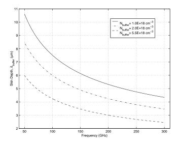
Figure 2.9: Plot of skin depth in the buffer layer vs. frequency for three doping levels.
