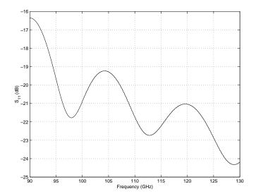
Figure 2.21: Plot of  $S_{11}$  for the WR-8 one-fifth to full height waveguide linear taper (simulated).
