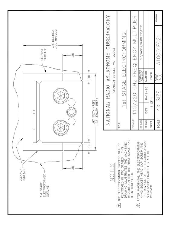
Figure D.30: 110/220 GHz frequency doubler: Details of the machining needed after completion of the first stage of electroforming.
