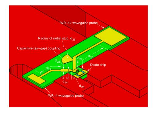
Figure 4.36: Design of the input and output embedding circuits. All the dimensions that were optimized are marked. The design of the 50  $\Omega$  microstrip to waveguide transition for both the input and output was carried forward from the previous block. Consequently, dimensions corresponding to those transitions did not need to be optimized. Only bottom half of the mount that seats the circuits is shown.
