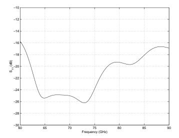
Figure 4.15: Plot of  $S_{11}$  for the input WR-12 waveguide to 50  $\Omega$  microstrip transition (simulated).
