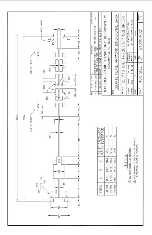
Figure B.2: Dimensional details of the artwork representing the metalization pattern on an individual quartz circuit used in the 55/110 GHz frequency doubler.
