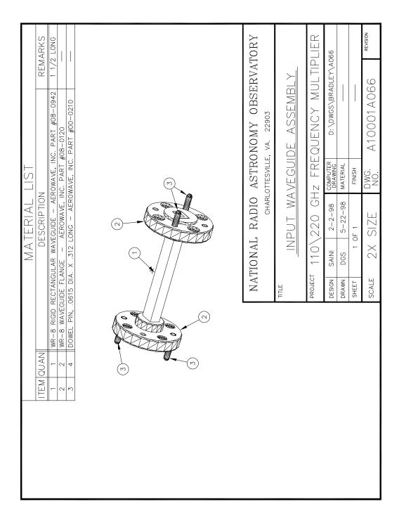
Figure D.18: 110/220 GHz frequency doubler: WR-8 input waveguide flange adapter assembly.
