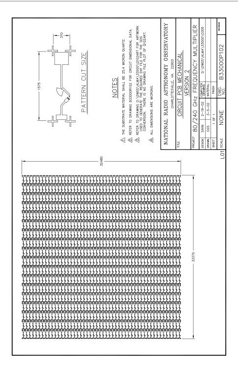
Figure B.6: Details of the mask set used in the fabrication of quartz circuits for the 80/240 GHz frequency tripler (version 2).
