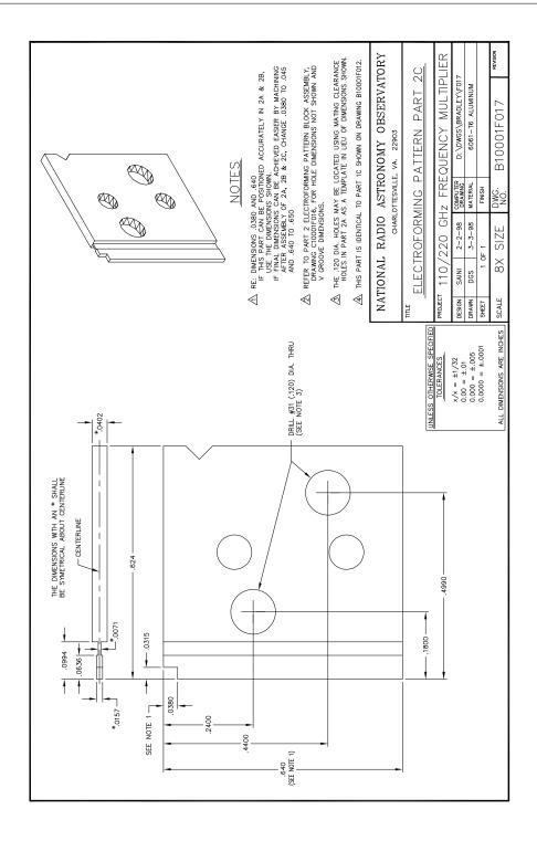
Figure D.28: 110/220 GHz frequency doubler: Mechanical details of the mandrel part 2C.
