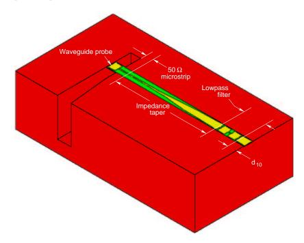
Figure 4.19: The complete input embedding circuit consisting of a waveguide to microstrip transition, a microstrip impedance taper and a lowpass filter. Only the bottom part of the mount that seats the quartz circuit is shown. The length of the section marked  $d_{10}$  was optimized such that the impedance presented to the
