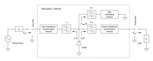
Figure 4.1: A single diode based frequency tripler.
