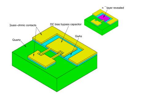
Figure 4.5: Layout of the quartz based integrated device, consisting of two Schottky diodes in an anti-parallel configuration and a large capacitor to accommodate the DC bias arrangement. The smaller inset is a view with the top metalization of capacitor removed to reveal the  $n^-$  layer underneath.
