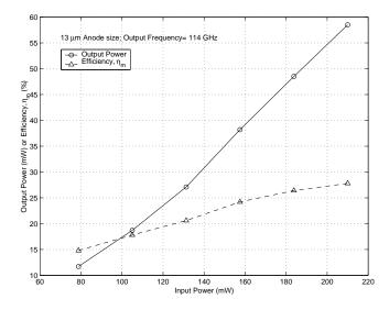
Figure 2.28: Measured output power and efficiency versus input pump power for an output frequency of 114 GHz.
