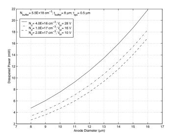
Figure 2.11: Power dissipated (per diode) under conditions of optimum operation for different anode sizes and epitaxial layer doping level.
