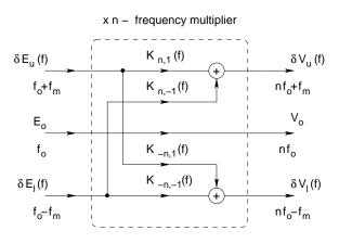
Figure 5.1: Transmission of sideband noise through a frequency multiplier, considered as a linear frequency converter.
