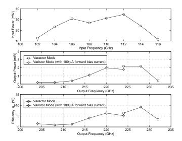
Figure 2.40: Measured performance of the 110/220 GHz frequency doubler, built using a diode array having anodes with 8  $\mu m$  diameter.
