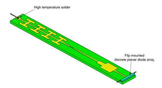
Figure E.3: Diagram of the quartz circuit after completion of the assembly procedure.
