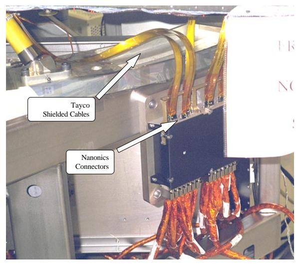
Figure 1 Nanonics Dualobe connectors attached to shielded twisted pair cables
