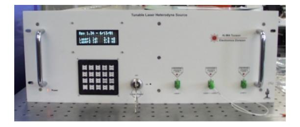
Fig. 3: Photograph of the front panel of the NRAO dual 1.55  $\mu$ m laser source. A keypad allows the user to set a difference frequency in the range from 1 GHz to 625 GHz
