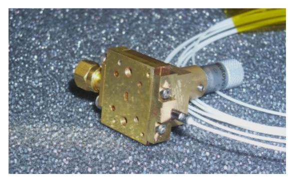
Fig. 2: Photograph of completed photonic sources showing theWR-10 output waveguide and the stainless steel fibre ferrule cemented to the block. The block base dimensions are 20 mm x 25 mm.
