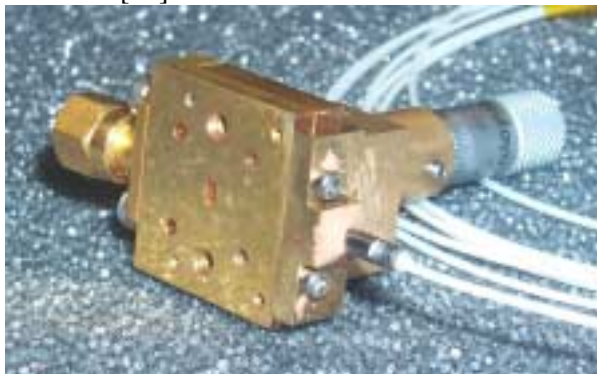
Figure 3 – W-band photomixer in 75-110 GHz frequency band.
