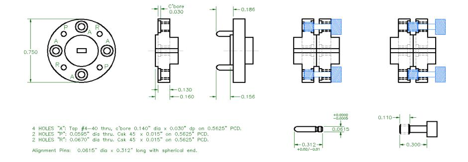
Fig. 1 The standard Mil-F-3922/67B flange with its raised central boss. The right hand diagrams show a pair of flanges engaged with the screws inserted and withdrawn.
