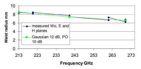
Fig. 3. Beam waist radii determined from the near-field measurements.
