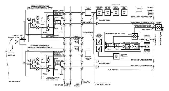
Fig. 1. Block diagram of cartridge.
