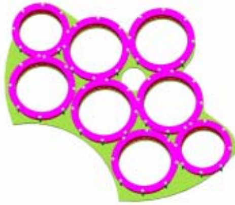
Figure 6-12: Distribution of thermal links on the 4K base plate A similar arrangement is used for the radiation shield links
